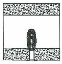
CMU and Terracotta Block Epoxy Anchor see Table 5, page 16 for anchoring details
